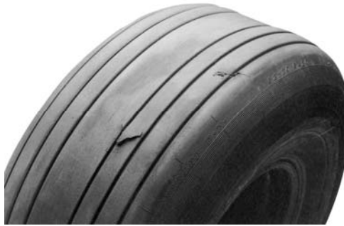
Cut Damage Figure 303
