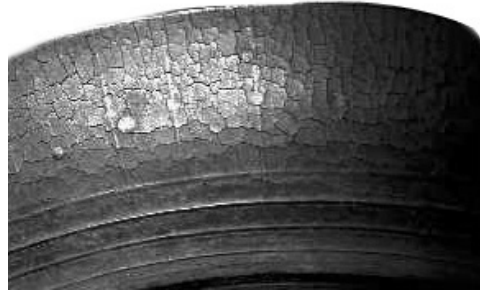
Sidewall Cracking Figure 310
